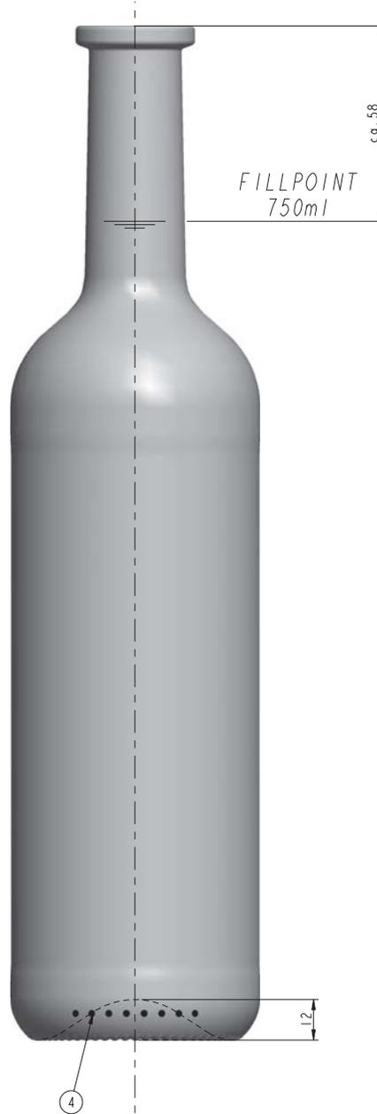
This detail only serves for the approximation of the attitude of the filling machine, the brimfull capacity remains binding
